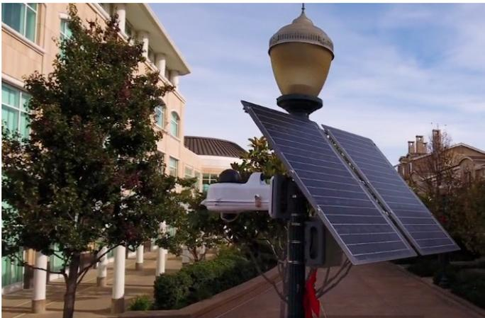
City leaders found a local company, called V5 Systems, which could solve all of the security challenges it faced. Its portable, self-powered security units could be rapidly deployed and moved anywhere. A unit could be taken down and put up again in minutes. As a result, the technology could be used to secure the downtown area, as well as remote infrastructure, without the huge costs and delays involved for permitting and trenching.
